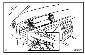
(c) Install the 2 bolts to hold the front passenger airbag assembly and instrument panel reinforcement.
