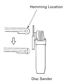
After grinding off the hemming location, remove the outer panel.
