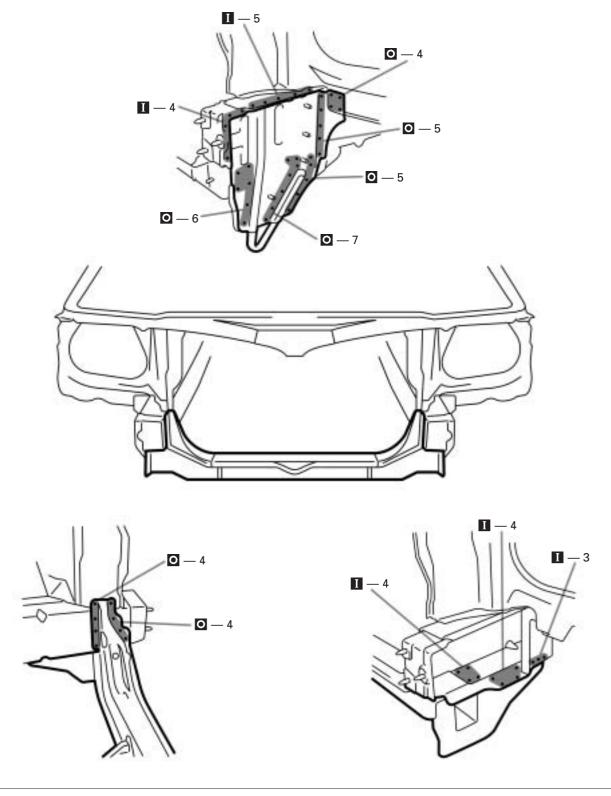
Temporarily install the new parts and measure each part in accordance with the body dimension diagram.
