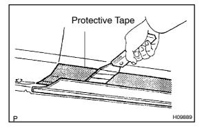
(c) Using a scraper, break the No.3 outside moulding clips and slowly remove the rocker panel moulding while separating attached part with the adhesive tape.
