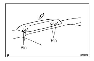
(c) Pull the center stop light assembly towards the front of vehicle to disconnect the four pins, disconnect the connector and remove the center stop light assembly.
