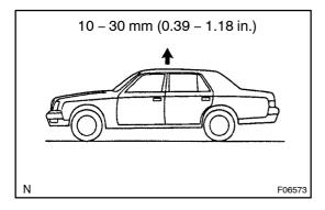
(c) Start the engine and set the height control switch from the "NORM" position to the "HIGH" position.
