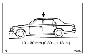
(d) With the vehicle height in "HIGH" position and the engine running, set the height control switch from the "HIGH" position to the "NORM" position.
