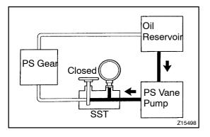
(f) With the engine idling, close the valve of the SST and observe the reading on the SST.
