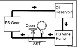
With the engine idling, open the valve fully. (g)
