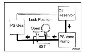
With the engine idling and valve fully opened, turn the (i) steering wheel to full lock.
