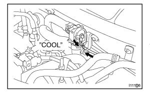
(d) Set the water valve lever on "COOL" position, connect the control cable and lock the clamp.
