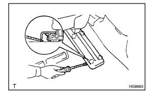
(c) Using a screwdriver, pry out the 2 front seat track covers. HINT:
