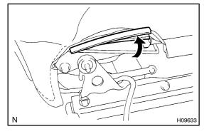
(c) Disengage the hook of the seat cushion cover.
