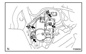
(d) Remove the 3 bolts, 2 nuts and the height control compressor and dryer with the bracket.
