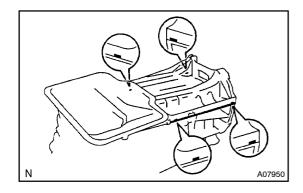
(b) Remove oil pan No.1 by prying off the points shown in the illustration with a bladed screwdriver.
