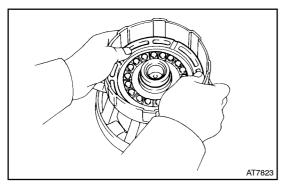
(b) Be careful not to damage the O-rings, press the clutch piston into the forward clutch drum with both hands.
