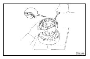
Using a screwdriver, install the snap ring.
