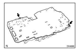
(d) Turn over upper valve body, remove the 2 screws and assembled gasket & plate.
