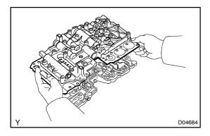
(b) Remove the upper valve body with the assembled gasket & plate.
