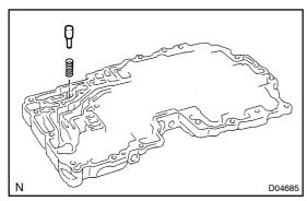
(c) Remove the check valve and spring from the lower valve body.
