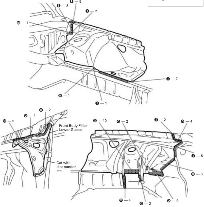
1. After removing the front body pillar lower gusset, remove the front fender apron.
