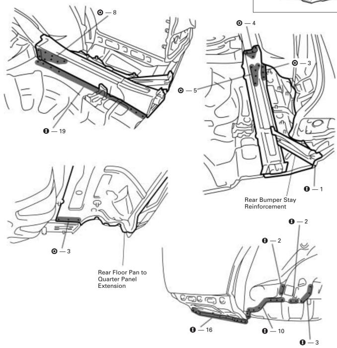
1. Replace the rear floor pan to quarter panel extension and rear bumper stay reinforcement at the same time.
