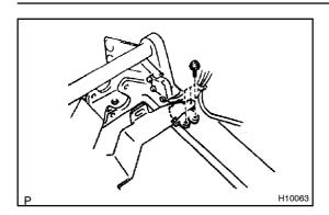
(b) Remove the 3 screws and limit switch.
