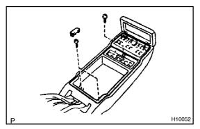
$\hbox{(k)} \quad \hbox{Using a screwdriver, remove the 2 covers.}$
