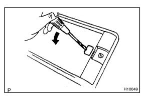
(f) Using a screwdriver, remove the cover from the center armrest door.
