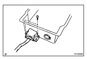
(o) Remove the 2 screws and microphone amplifier assembly.
