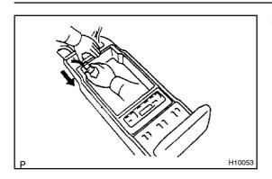
(j) Remove the power outlet socket as shown in the illustration.
