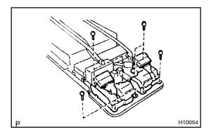
(m) Remove the 8 screws and power seat switch assembly.
