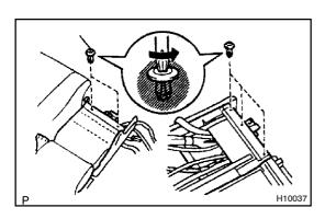
(b) Remove the 5 clips and center armrest assembly.
