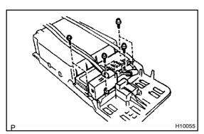
(n) Remove the 6 screws and switch & volume assembly and courtesy light switch.
