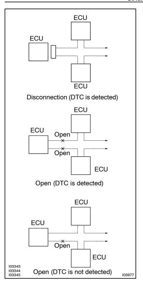
(b) If DTC of ECU communication stop is output, there is a possibility of connector disconnection or 2 communication buses open. It will not become abnormal with only 1 communication bus open.
