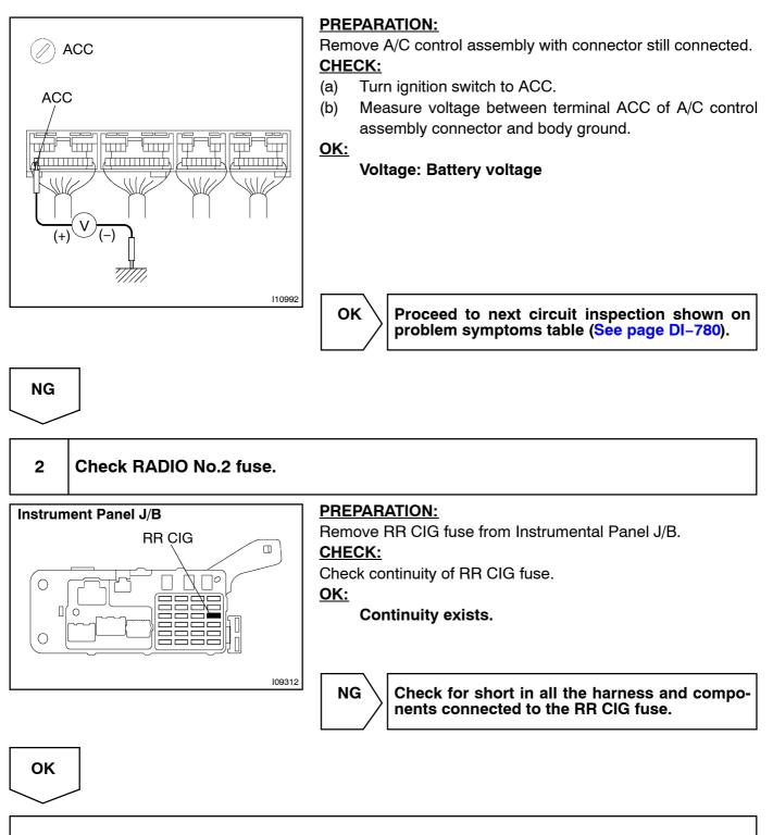
Check and repair harness and connector between A/C control assembly and battery.
