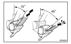
(d) Make sure that the belt can be pulled out at a tilt of 15 degrees or less, and cannot be pulled out over 45 degrees of tilt.
