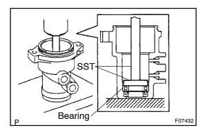
(d) Using SST, press in a new bearing. SST 09950-60010 (09951-00340), 09950-70010 (09951-07150)
