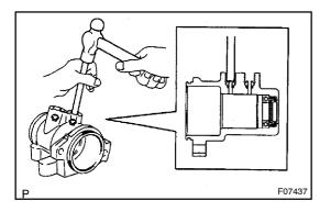
(b) Using a plastic hammer and sliding handle, lightly tap in a new union seat.
