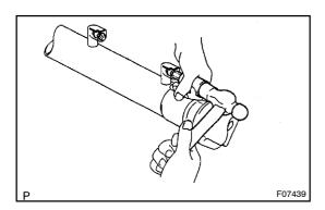
(b) Using a socket hexagon wrench (8 mm) and a hammer, lightly tap in a new union seat.
