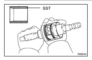
(f) Carefully slide the tapered end of SST over the rings until they fit to the control valve assembly.
