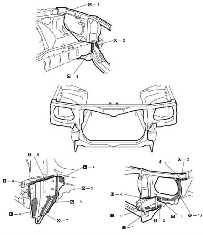
Temporarily install the new parts and measure each part in accordance with the body dimension diagram.
