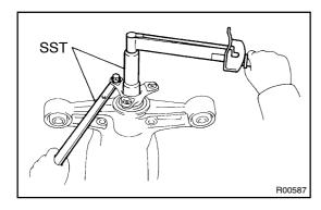
If the preload is greater than the specified value, replace the bearing spacer.
