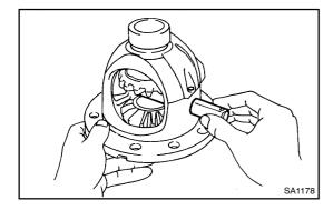
(b) Install the 2 side gears, pinion gears, pinion gear thrust washers and pinion gear shaft in the differential case.
