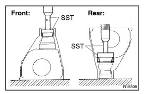
(a) Using SST and a press, install the front bearing outer race.
