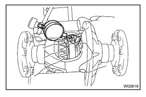
(d) Using a dial indicator, measure the pinion gear backlash while holding one side gear toward the case.
