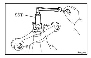
(c) Using SST and a torque wrench, measure the preload.
