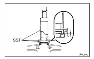
(b) Using SST, install the oil seal until its end is flush with the differential carrier.
