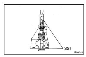
(b) Using SST and a press, install the front bearing on the drive pinion.
