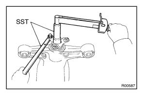
(b) Using SST, tighten the nut. SST 09229-55010, 09330-00021
