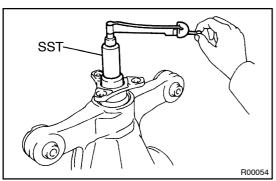
(c) Using SST and a torque wrench, measure the preload. SST 09229-55010
