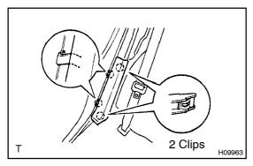
(d) Using a screwdriver, remove the rear side seatback. HINT:
