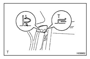
(b) Using a screwdriver, remove the rear seatback stay cover. HINT:
