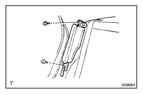
(e) Disconnect the connector, then remove the 2 bolts and rear seat side airbag.
