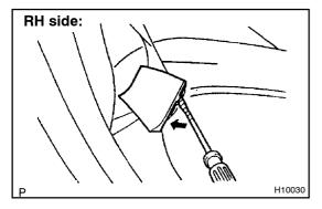
(b) Using a screwdriver, open the belt protectors, then remove the rear seat outer belts by pulling off.
