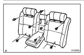
(c) Remove the 8 bolts, 2 nuts and seatback assembly, then disconnect the connector.
