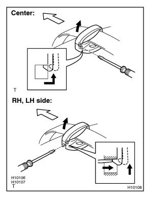
(b) Using a screwdriver, remove the rear seat belt from the rear seat shoulder belt guide as shown in the illustration.
