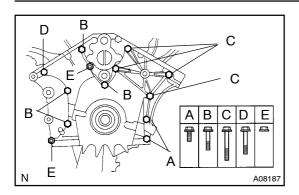
(c) Install the chain cover with 11 bolts and 2 nuts.
