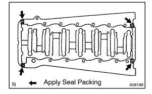
(b) Apply seal packing (3 – 5 mm width) to the positions shown in the illustration on the cylinder block.
