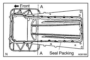
(c) Apply seal packing to the positions shown in the illustration continuously in bead form (2 – 3 mm width) and install the cylinder block.
