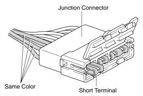
Junction connector in this manual include a short terminal which is connected to a number of wire harnesses. Always perform inspection with the short terminal installed. (When installing the wire harnesses, the harnesses can be connected to any position within the short terminal grouping. Accordingly, in other vehicles, the same position in the short terminal may be connected to a wire harness from a different part.)
