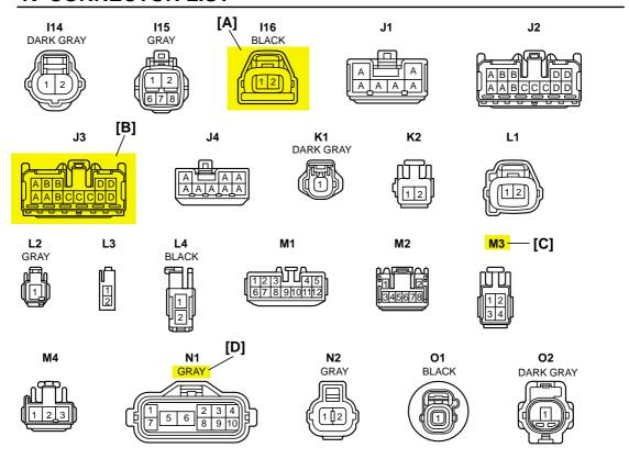
[A]: Indicates connector to be connected to a part. (The numeral indicates the pin No.)
