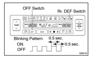
(2) If mode indication is different from the actual air outlet in actuator check, turn ignition switch to ON or START while pressing "Rr DEF" and "OFF" switches simultaneously. Step motor initialization occurs and the "DEF" indicator blinks.
