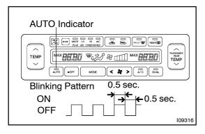
(b) Step motor initializing procedure (Compulsory initializing).
