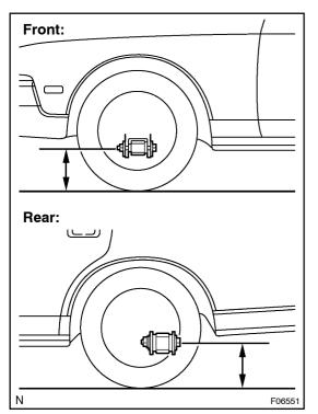
(g) When the radius of a tire is 308 mm (12.13 in.) vehicle height will be the value described in the chart below.
