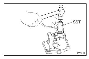
(b) Using SST and a hammer, drive out the bearing. SST 09325-12010
