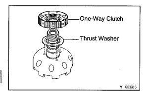
3. REMOVE ONE — WAY CLUTCH AND THRUST WASHER FROM SUN GEAR INPUT DRUM
