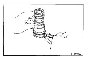
5. REMOVE SNAP RING FROM PLANETARY SUN GEAR
