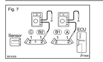
(2) Disconnect connector "B" and measure the resistance between terminal 1 of connector "A" and body ground, and terminal 1 of connector "B2" and body ground.
