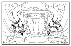
(b) Install the 2 catalytic converter supporting brackets with the 4 bolts.
