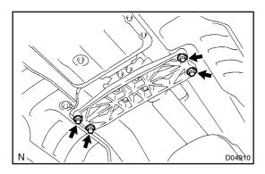
5. INSTALL 4 ENGINE REAR MOUNTING SET BOLT Torque: 26 N·m (265 kgf·cm, 19 ft·lbf)
