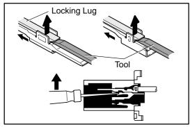
(c) Release the locking lug from terminal and pull the terminal out from rear.
