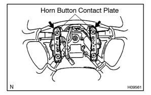
• Check the deformation of the horn button contact plate on the steering wheel.
