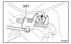
(b) Raise the differential carrier with a jack and install the 2 lower mount stoppers and new bolts.
