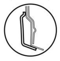
1. Cut and join the part at the location (near the center of vehicle) as shown above.
