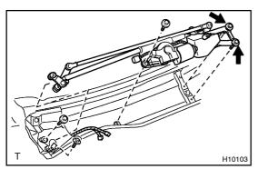
6. REMOVE WIPER MOTOR AND LINK ASSEMBLY
