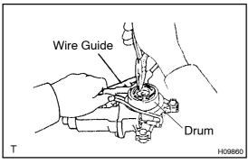
(b) Using needle nose pliers, remove the drum and wire guide from the motor.
