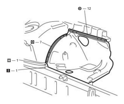
Temporarily install the new parts and measure each part in accordance with the body dimension diagram.
