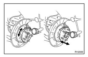
(e) Using a dial indicator, check the backlash near the center of the axle hub.
