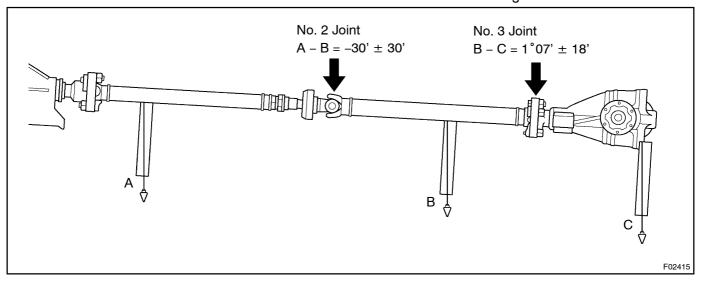
If the measured angle is not within the specified value, adjust it with the center support bearing adjusting washer.
