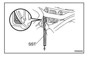
(b) Using SST, measure the installation angle of the differential.
