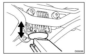
(b) Using a jack, raise and lower the differential to stabilize the differential mounting cushion.
