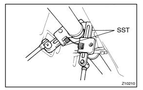
(i) Using SST, tighten the adjusting nut. SST 09922-10010
