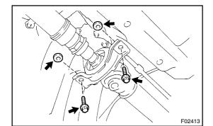
(c) Temporarily install the 2 center support bearing set bolts with the adjusting washers.
