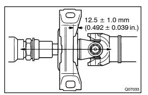
(h) Torque the 2 center support bearing set bolts.
