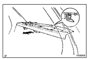
(b) Remove the package tray trim board as shown in the illustration.
