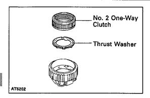
(c) Remove No.2 one—way clutch with retainers and No. 2 thrust washer from the planetary gear.
