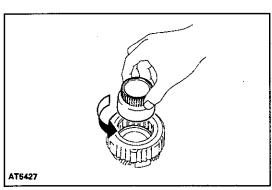
(c) While turning it counterclockwise, install the one—way clutch inner race to the rear planetary gear.
