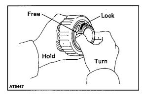
4. CHECK OPERATION OF NO.2 ONE—WAY CLUTCH Hold the planetary gear and turn the one—way clutch inner race. The one—way clutch inner race turns freely counterclockwise and locks clockwise.
