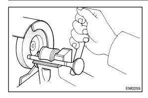
(c) Check the surface of the valve stem tip for wear. If the valve stem tip is worn, resurface the tip with a grinder or replace the valve.
