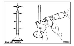
Using a micrometer, measure the diameter of the valve (b) stem.
