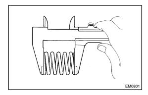
(b) Using vernier calipers, measure the free length of the valve spring.
