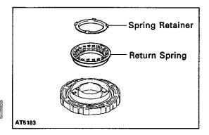
(c) Remove the spring retainer and return spring.
