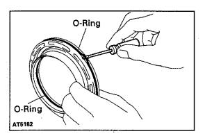
(c) Remove the 2 O-rings from the piston.
