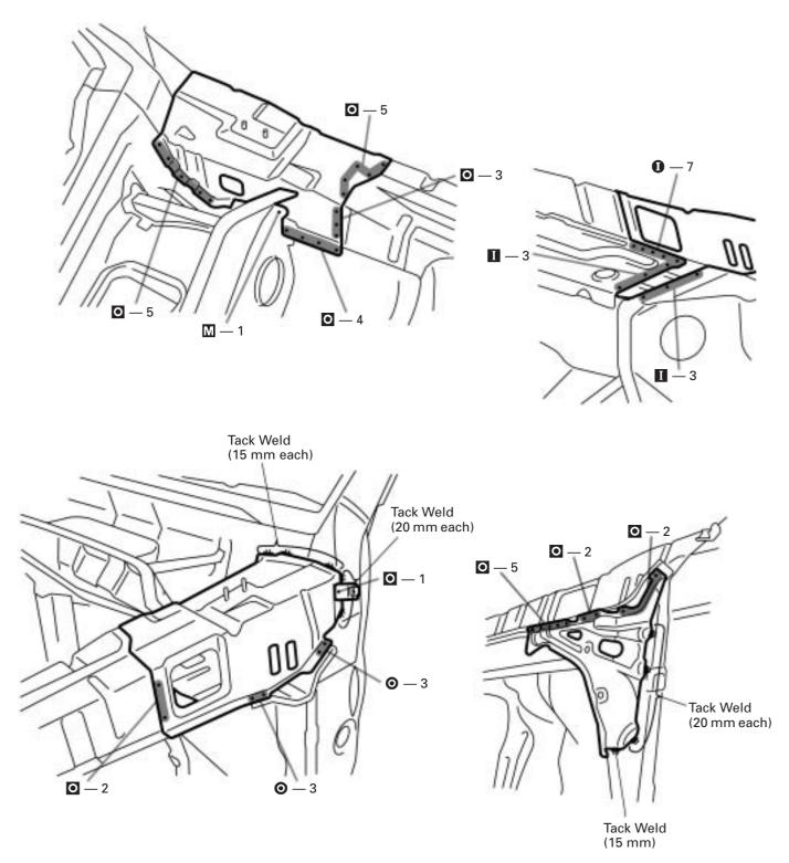
1. Temporarily install the new parts and measure each part accordance with the body dimension diagram.
