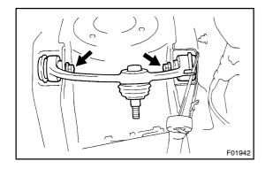
(b) Remove the 2 bolts and the upper suspension arm.
