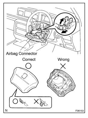
(d) Pull out the wheel pad from the steering wheel and disconnect the airbag connector.
