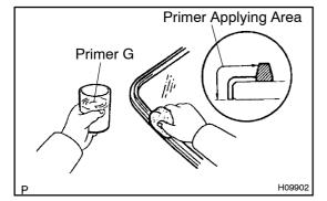
9. COAT CONTACT SURFACE OF BODY WITH PRIMER "M"
