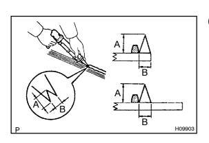
(c) Coat the glass with adhesive as shown.
