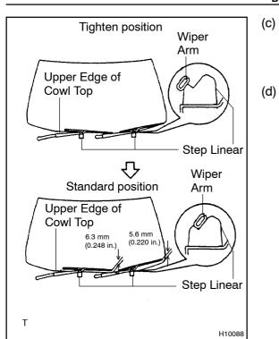
(c) Move the wiper arms from the step linears, slightly slide downwards to align the tip of blade with the upper edge of cowl top, and tighten nuts.
