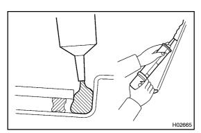
14. APPLY ADHESIVE TO MOULDING INSTALLATION AREA
