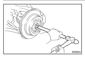
(f) Using a brass bar and hammer, lightly tap the end of the drive shaft to disengage the axle hub and remove the drive shaft.
