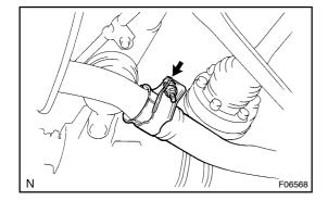
(b) Loosen the bolt and remove the tailpipe.
